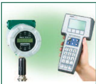
VorTek Instruments' Pro-V™ multivariable flowmeters utilize three primary sensing elements—a vortex shedding velocity sensor, an RTD temperature sensor, and a solid-state pressure transducer—to measure the mass flow rate of gases, liquids and steam. Because the Pro-V™ is able to measure all process variables within a single device it provides exceptional accuracy, simplifies system design and reduces installation costs.
